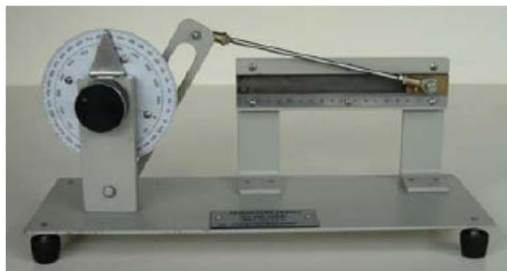
Figure 5.3-1: Slotted link mechanism: apparatus and schematic.
