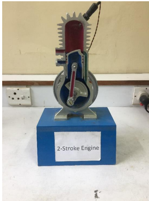
Figure 1: Sectioned model of a two-stroke engine
