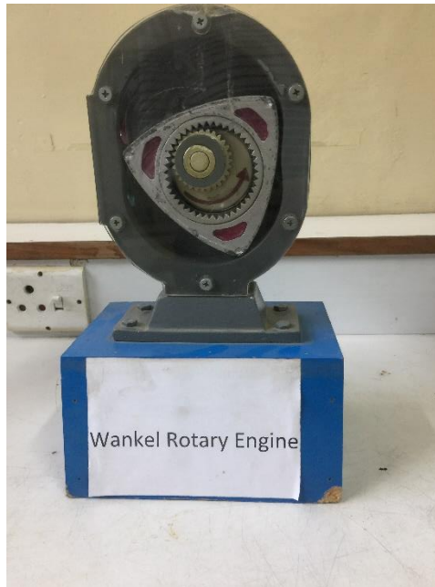
Figure 5: Sectioned model of a Wankel engine
