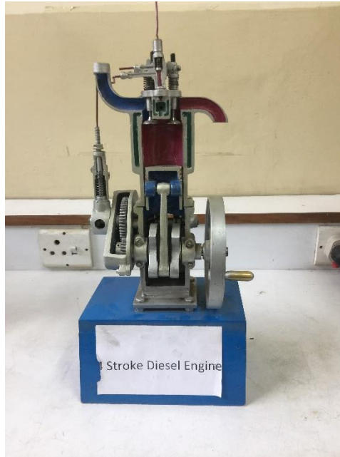
Figure 3: Sectioned model of a four-stroke engine diesel engine
