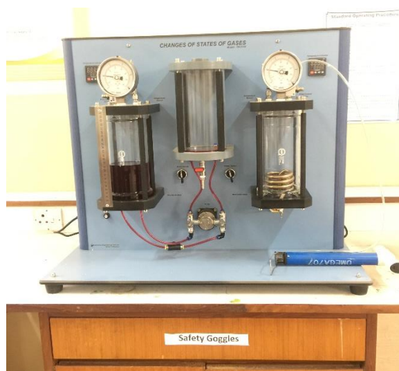
Figure 12: Experimental setup for Boyle's law and Gay-Lussac's law
