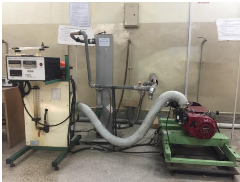
Figure 10: Exhaust gas calorimeter
